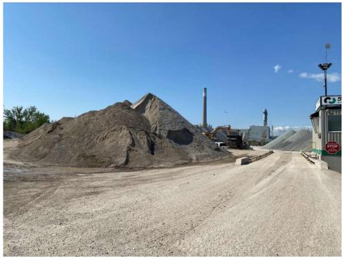
Photo (33): Strada Aggregate Crusher: 10 Leslie St, Toronto, ON – Stockpiles of RCA
