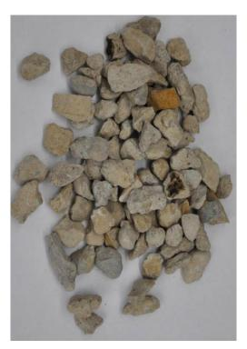
Figure 11. Photo of Recycled Concrete Aggregate (RCA) Obtained from Concrete Pavements [12]
