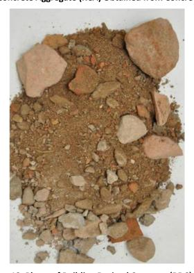
Figure 12. Photo of Building Derived Concrete (BDC) [12]
