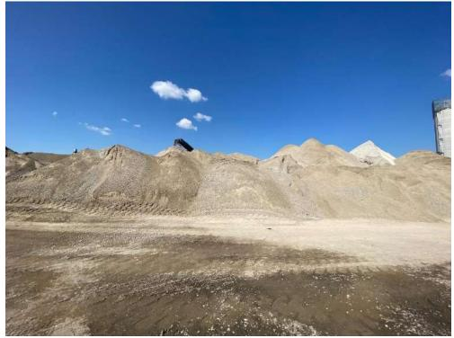
Photo (32): Strada Aggregate Crusher: 10 Leslie St, Toronto, ON – Stockpiles of RCA (Gran A RAP)
