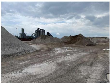
Photo (15): Crupi Crusher at 2777 14th Ave, Markham-Stockpiles of Produced RCA and RAP
