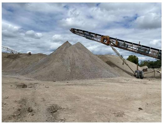
Photo (27): Strada Aggregate Crusher: 120 Wentworth Crt, Brampton, ON – Stockpiling of RCA
