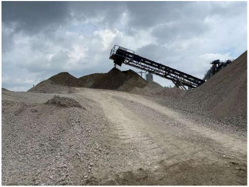
Photo (14): Crupi Crusher at 2777 14th Ave, Markham-Stockpiling of Produced RCA
