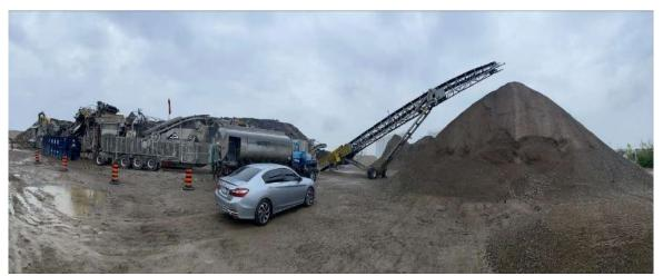
Photo (17): Crupi Crusher at 176 Bethridge Rd, Etobicoke, ON – Producing RCA
