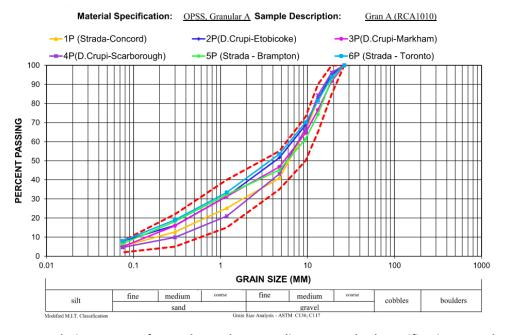
Figure 46: Gradation Curves of Tested Samples According to Standard Specifications Envelope
