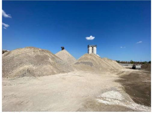
Photo (30): Strada Aggregate Crusher: 10 Leslie St, Toronto, ON- Stockpiles of RCA
