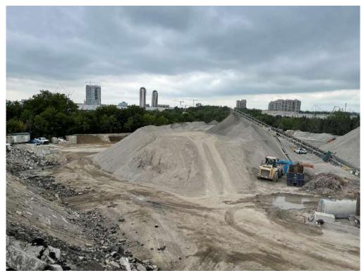
Photo (9): Strada Crusher at 1667 Creditstone Rd, Concord, ON – Stockpile of RCA (Gran A RAP)
