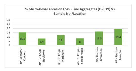
Figure 50: Histogram for % Micro-Deval Abrasion Loss (for fine aggregate) of Tested Samples
