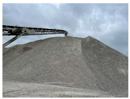
Photo (8): Strada Crusher at 1667 Creditstone Rd, Concord, ON – Stockpile of RCA (Gran A RAP)
