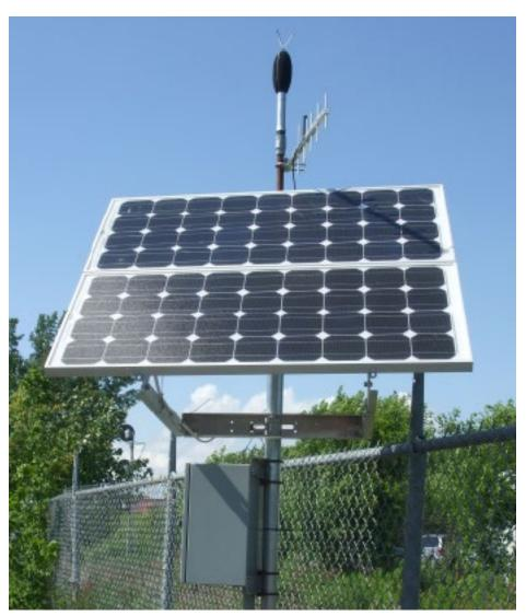
A real-time monitoring station allows operators to modify site operations proactively to reduce noise
